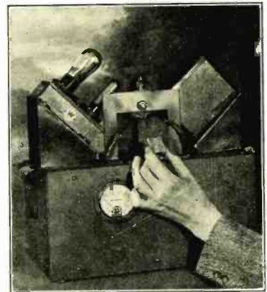
Fig. 14. Sorting small packages for imperfect labels by means of photoelectric tube.
